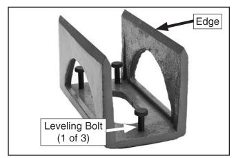
Figure 30. Wheel balancing base.
